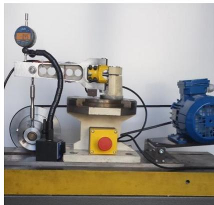
Fig. 1. Strain controlled stand for bending loading
