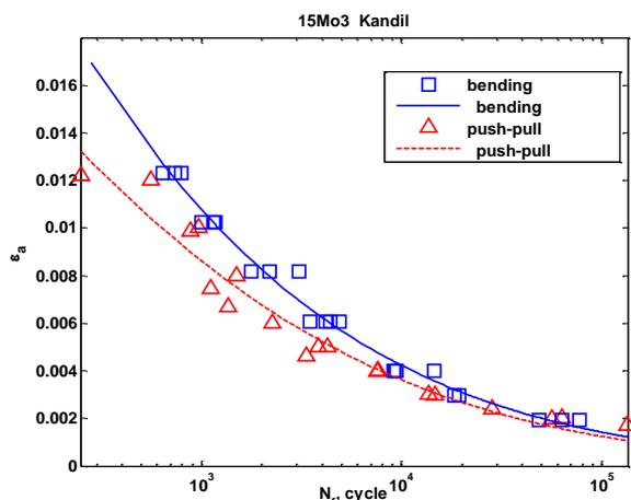
Fig. 6. Strain-life curves according to Kandil's model for both push-pull and bending tests
