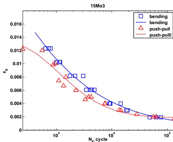
Fig. 8. Strain-life curves according to Author's model
