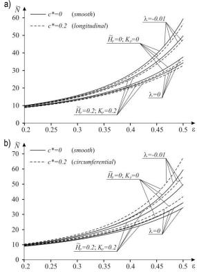
**Fig. 6.** Load-carrying capacity for the squeeze film thrust bearing with rough surfaces for  $\widetilde{H}_p = 0.2$ ,  $K_p = 0.2$ ,  $\lambda = -0.01$  and  $\lambda = 0$  and  $\varepsilon = 0.5$ ; (a) longitudinal roughness and (b) circumferential roughness
