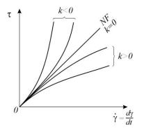
**Fig. 1.** Flows curves of a Rotem-Shinnar fluid of the first order (i = 1); symbol NF means a Newtonian fluid
