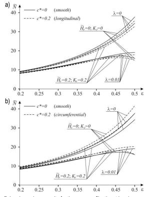
**Fig. 7.** Load-carrying capacity for the squeeze film thrust bearing with rough surfaces for  $\widetilde{H}_p = 0.2$ ,  $K_p = 0.2$ ,  $\lambda = 0$  and  $\lambda = 0.01$  and  $\varepsilon = 0.5$ ; (a) longitudinal roughness and (b) circumferential roughness
