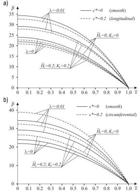
**Fig. 4.** Dimensionless pressure distribution in the squeeze film thrust bearing with rough surfaces for  $\tilde{H}_p = 0.2$ ,  $K_p = 0.2$ ,  $\lambda = -0.01$  and  $\lambda = 0$  and  $\varepsilon = 0.5$ ; (a) longitudinal roughness and (b) circumferential roughness
