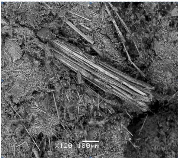
Figure 3 Chrysotile fibres on electronic microscope (magnification 120x)
