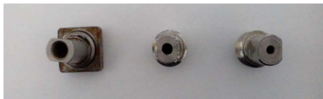
Figure 4. Replaceable heads of the screw press: (from the left), diameter \phi_3=6 mm), \phi_2=4 mm and \phi_1=2 mm
