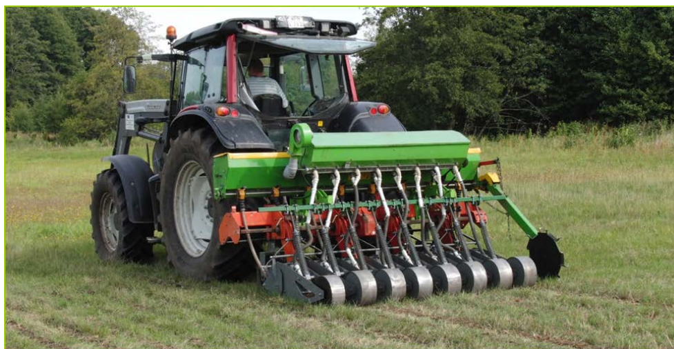
Figure 2. Wide-strip overseeding aggregate for grassland renovation (source: MAZOB-ITP, Khudzienko)
