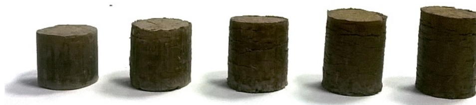
Figure 4. Samples of the obtained granulates (from the left A0 to A100) based on digestate from Piekoszów biogas plant
