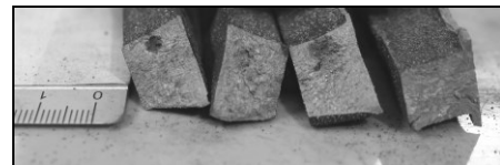
Fig. 4. Result of Althoff-Radtke test for sample modified 0.25% Fe-Ti; respectively, from the left arm length 50, 150, 250, 350 mm
