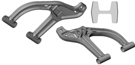
Fig. 5. Model configuration of the lower rocker arm with an I-shaped cross-section.
