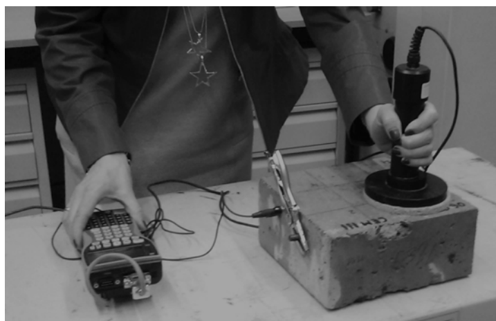
Fig. 1. Measurement on one of the tested specimens by the use of the galvanostatic pulse method
