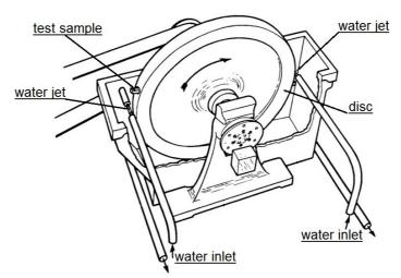
Fig. 3. Rotating disk-and jet repetitive impact apparatus, according to ASTM G 73 [27]
