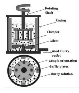
Fig. 6. Slurry pot test device [55]
