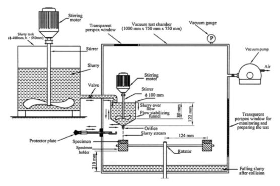
Fig. 8. Schematic diagram of whirling arm test device [63]
