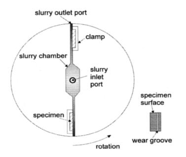
Fig. 7. Coriolis erosion tester [56]
