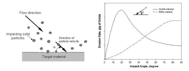
Fig. 1. Schematic of slurry erosion [13]
