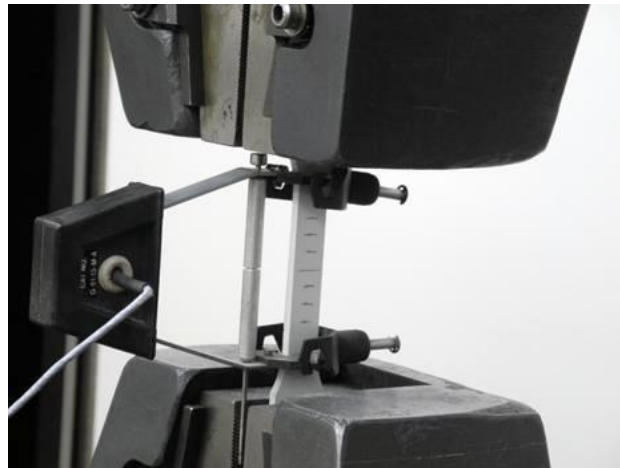
Fig. 1. Measurement of strain performed by extensometer on universal testing machine INSTRON
