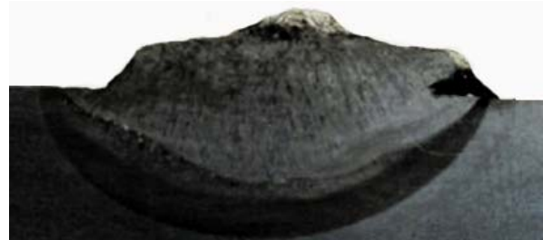
Fig. 3. Cross sections of weld beads: a) sample 5 - pitch 55%, b) sample 6 - pitch 89%, c) sample 7 - pitch 100%
