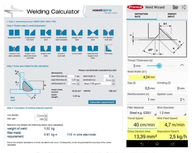
Fig. 4. Calculations performed in "Welding Calculator" and "Weld Wizard"
