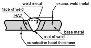
Fig. 1. Butt weld - scheme of welded joint
