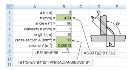
Fig. 3. Calculations performed in excel spreadsheet
