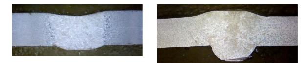
Fig. 2. Butt weld; a) non-alloyed steel, b) stainless steel
