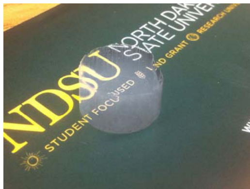
Fig. 6. Photograph showing an example of a transparent and crack-free silica aerogel in this study. The small piece of the aerogel missing was accidentally separated from the alcogel when it was removed from the mold
