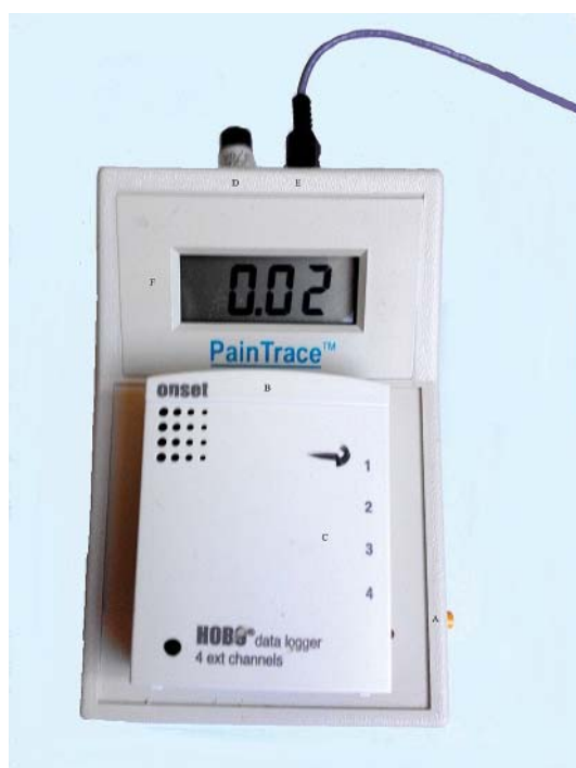
Figure 1. The Pain Trace™ device: A-on/off button; B-hobo data logger-box; C- four ports for connecting the logger to the device; D-amplifier port; E-cable port; F-display.
