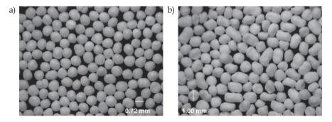
Fig. 2. a) Pellet images of formulation 3 (low acyl gellan gum, maltodextrin) and b) formulation 4 (PVP, Starch 1500<sup>®</sup>), with 1.18 and 1.44 aspect ratio values, respectively.
