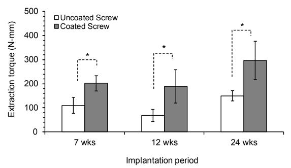
**Figure 4.** Extraction torque from bone of 12 uncoated and 12 coated titanium screws at different implantation periods (wks, weeks) (error bars, standard deviation, n = 4 per type per time point). \*P < 0.05
