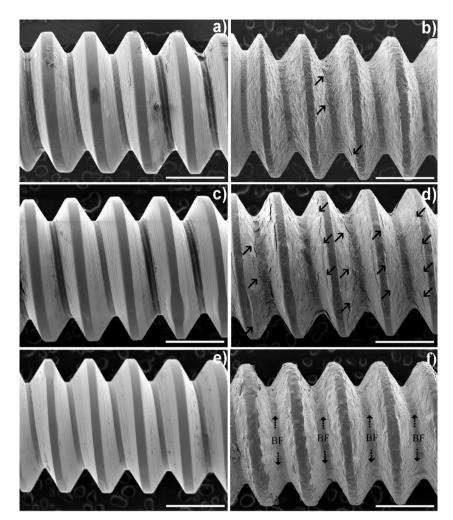
**Figure 5.** Scanning electron microscopy (SEM) image of uncoated and coated screws extracted from the bone. No detachment of the coating from the underlying screw is noted. Arrows indicate bone fragments (BFs). The amount and size of the BFs increased with increasing implantation periods. a) uncoated 7 weeks; b) coated 7 weeks; c) uncoated 12 weeks; d) coated 12 weeks; e) uncoated 24 weeks; and f) coated 24 weeks (magnification ×100). Scale bars represent 1 mm
