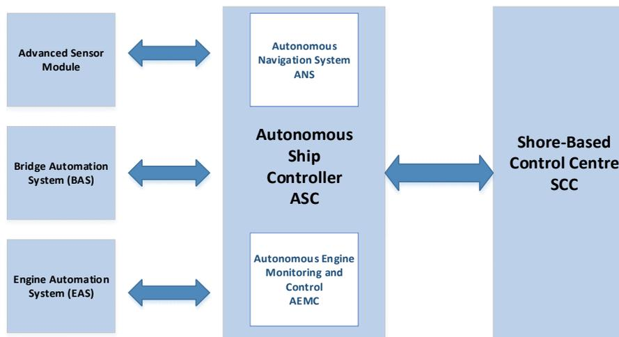
Figure 1: Overview of the autonomous ship modules (MUNIN, 2013)
