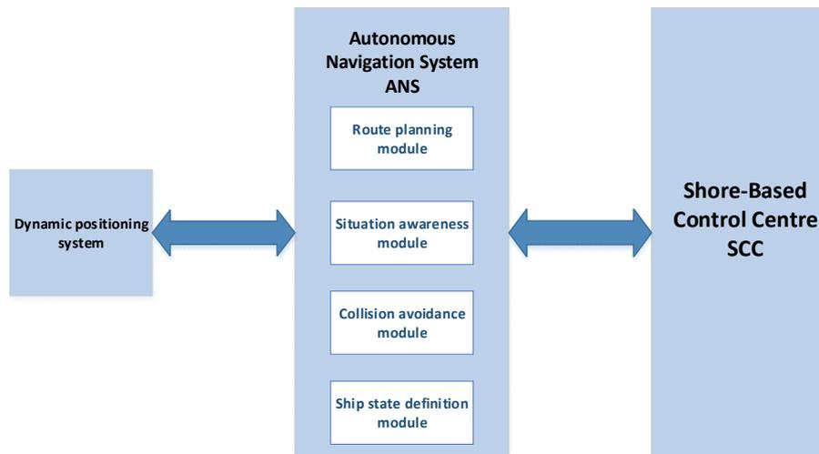
Figure 2: Autonomous Navigation System (ANS) architecture, (AAWA, 2016)
