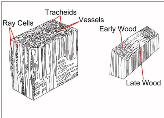
**Figure 21.2:** Macro-structural elements of wood (Source: Brodie 2008).
