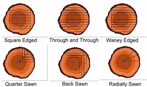
Figure 21.3: Various methods of sawing timber (Source: Brodie 2008).
