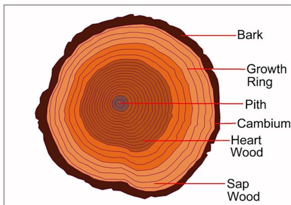
**Figure 21.1:** Cross section of tree trunk (Source: Brodie 2008).
