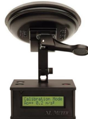
Fig. 3. Device XL metre used during measurements
