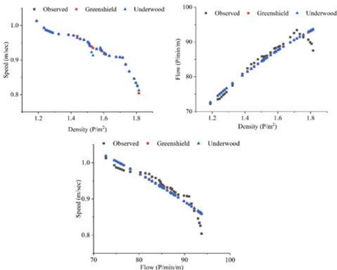
Figure 2. Crowd flow models: Speed–density model, Flow–density model, Speed–flow model
