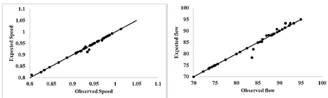
Figure 5. Observed and predicted speed and flow (ANN model): Observed and estimated speed, Observed and estimated flow
