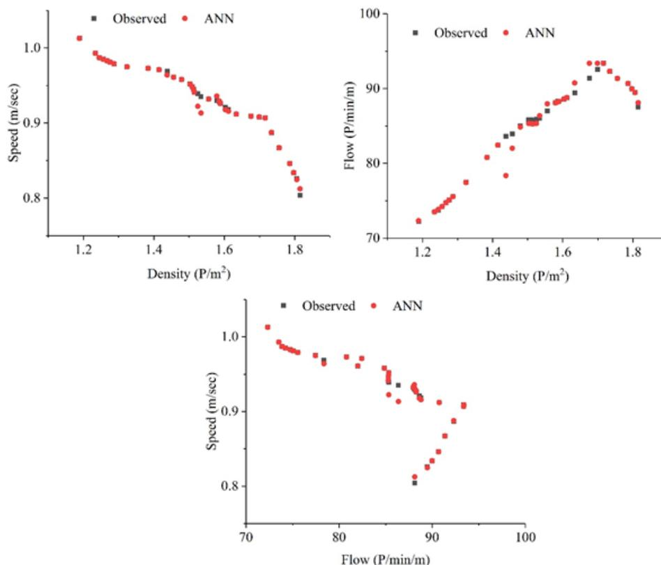
Figure 4. Crowd fundamental flow relationships using ANN. Speed–density model, Flow–density model, Speed–flow model
