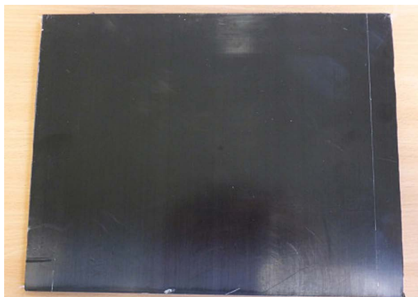
Fig.4. Cured composite panel [The Author 2016]
