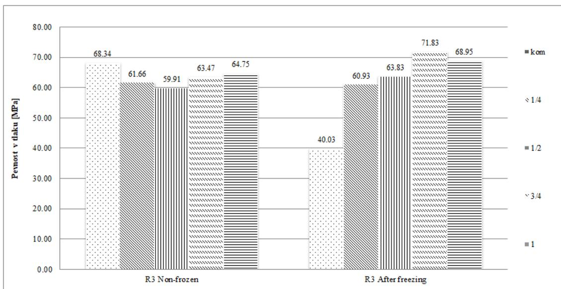
Figure 4: Compressive strengths of recipes R3
