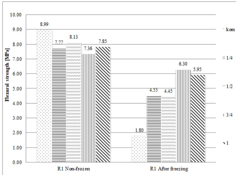
Figure 1: Flexural strength of R1 recipe
