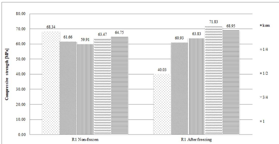
Figure 3: Compressive strengths of recipes R1
