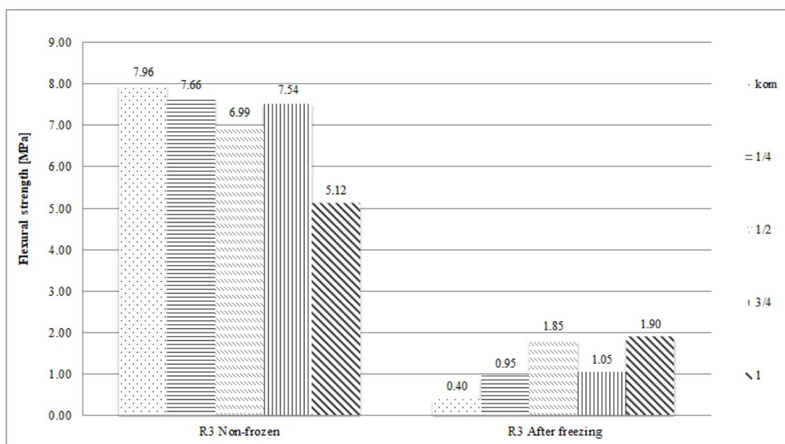
Figure 2: Flexural strengths of R3 recipe
