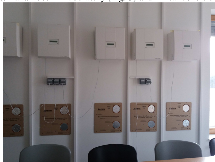
Figure 5: Laboratory stands for the study of in-wall ventilation units with heat recuperators in TTU
