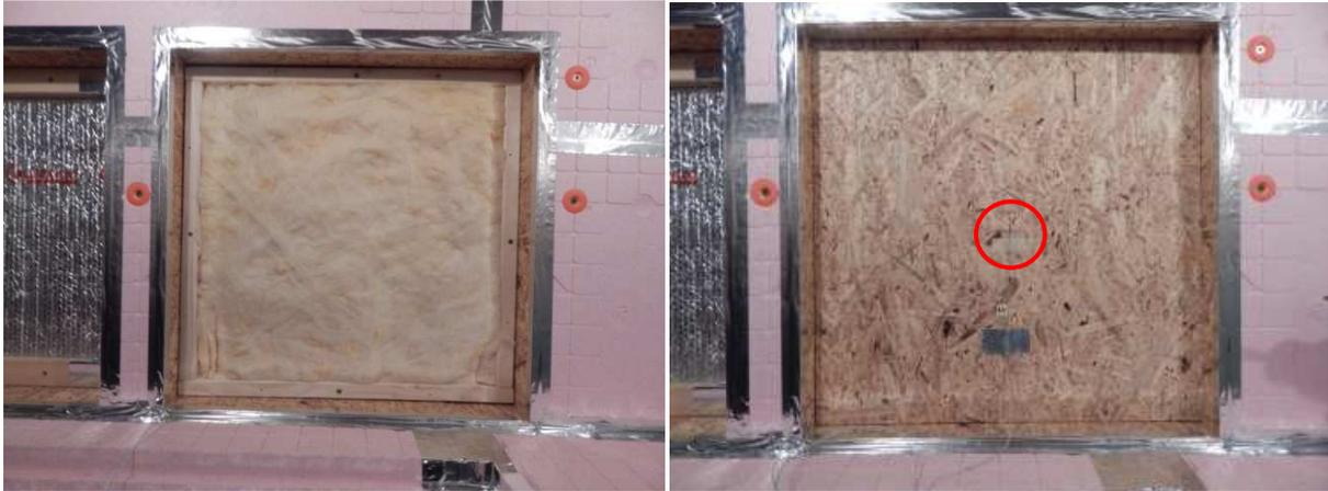
Figure 6: Inserting thermal insulation layer - mineral wool and installation sensor of surface temperature
