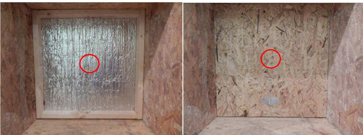
Figure 5: Location of the sensor of temperature in structure and surface temperature
