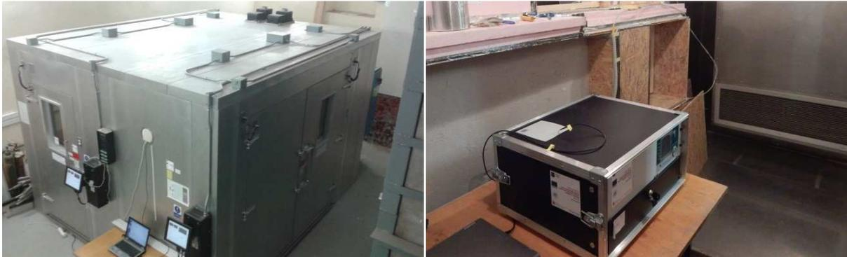
Figure 2: Climatic chamber and data logger Almemo 5690-1 connected to PC
