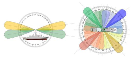
Fig. 3. Characteristics of the adaptive radiation of the antenna system
