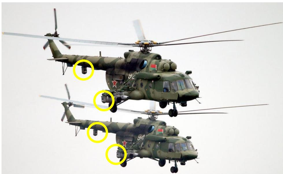
Fig. 14. Russian Mi-17 helicopters with the L370-5 system during exercises ZAPAD-2017 [21]
