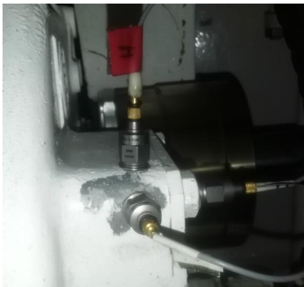
Fig. 6. Example of assembly of accelerometers on the reduction gear [author's photo]
