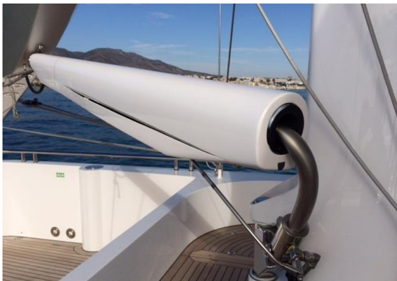
Fig. 3. Example the fracture in stormy conditions boom vang (kicking strap) [author's photo]
