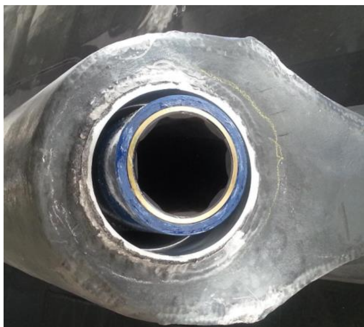
Fig. 4. The resin inner tube mounted into aluminum outer tub of shaftlines strut [author's photo]
