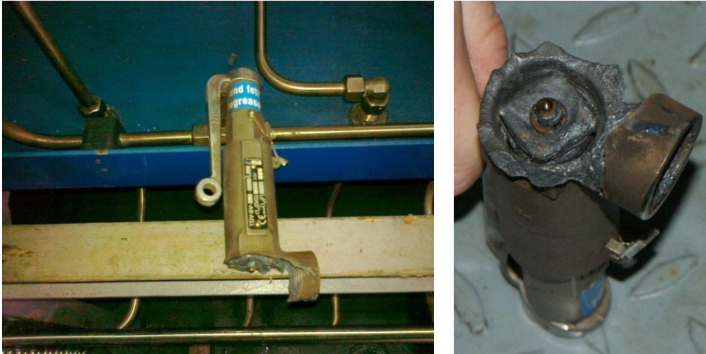
Fig. 1. Safety valve system of oxygen supply after oxygen ignition [PHU 'AQUATICUS', 2011] 8
