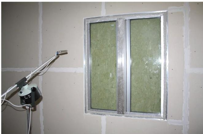
Fig. 14 Measured sample of the ventilation unit situated in the receiving room of the acoustic chambers
