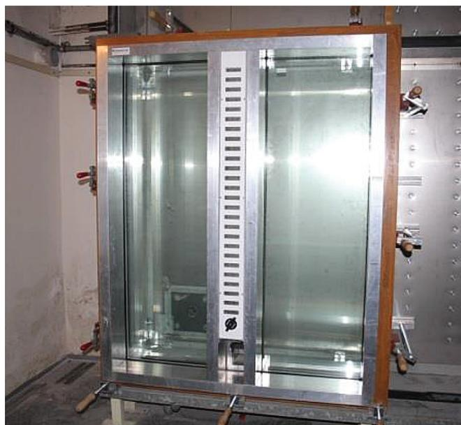
Fig. 11 View of the measured sample of the ventilation unit with the installed system of mechanically closable apertures in its inner zone fitted in the large pressure chamber
