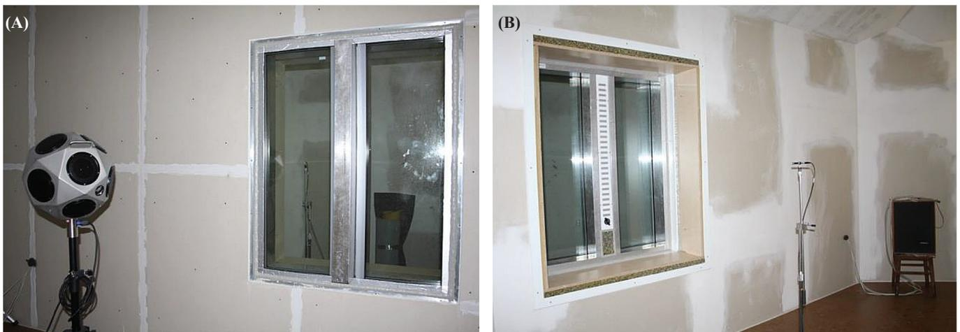
Fig. 15 Views from the source room (A) and the receiving room (B) to the measured façade element situated in the aperture of the partition of the acoustic chambers
