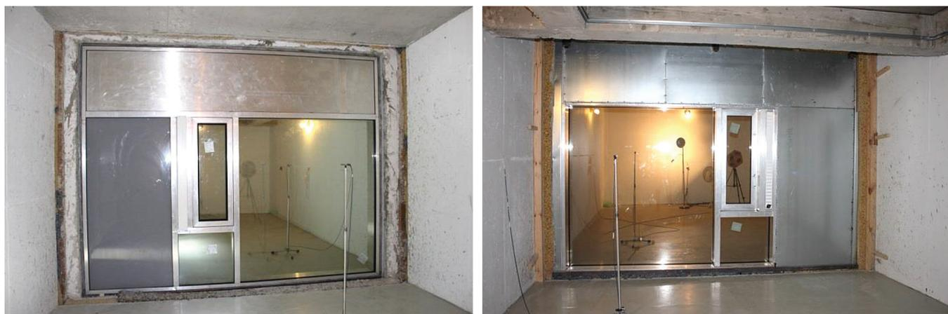
Fig. 19 Measured sample of the transparent facade element, view of the transmission rooms
