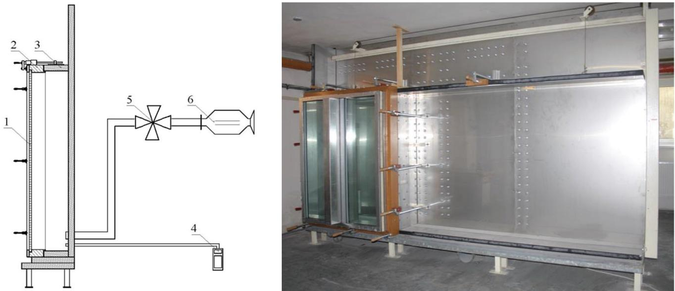
Fig. 12 Scheme of the large pressure chamber
