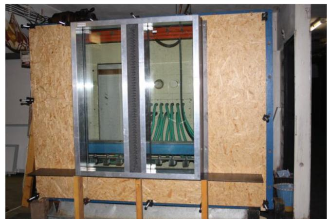
**Fig. 10** Overall view of the test sample placed in a large rain chamber
