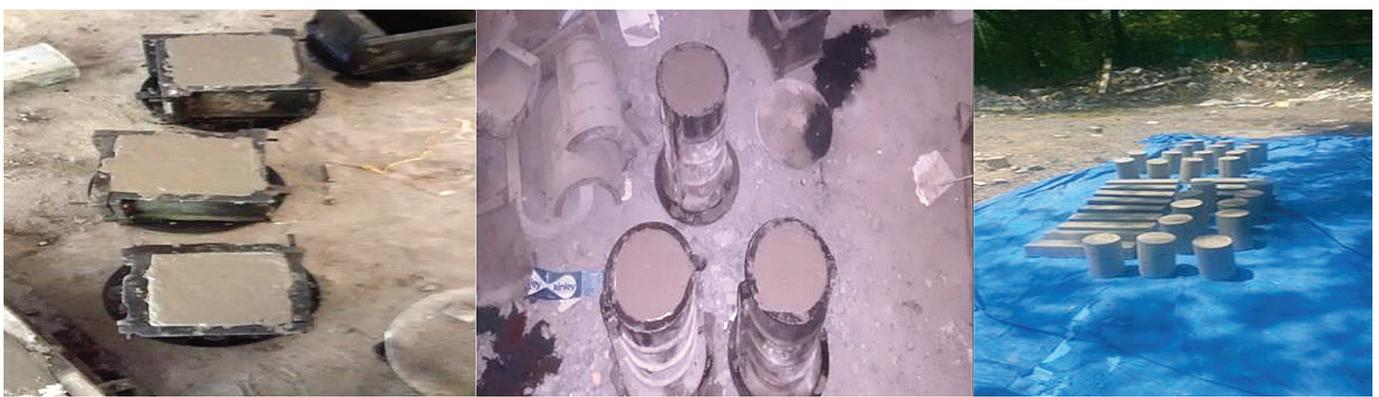
Fig. 1 Casting and curing of GPC specimens.
