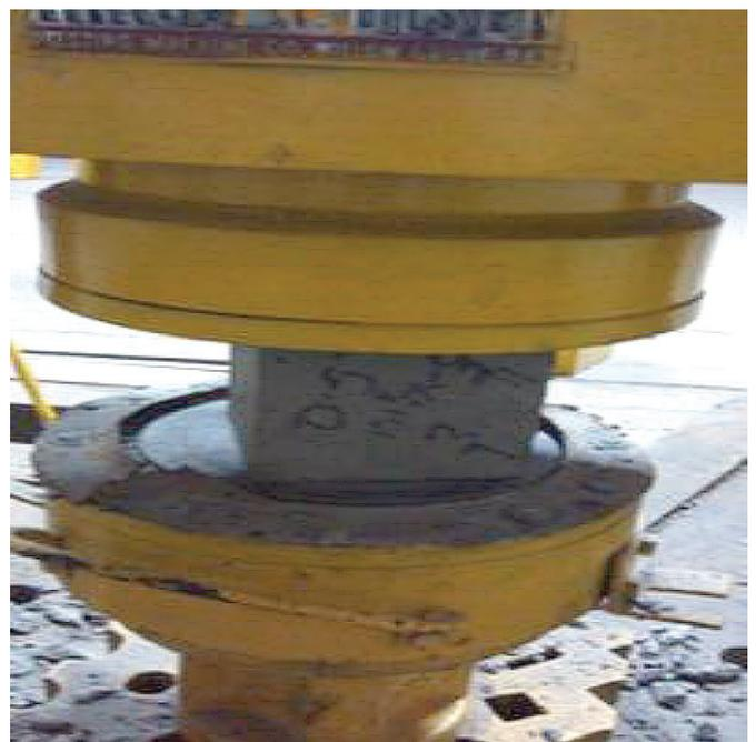
Fig. 3 Compressive Strength of Cube.
