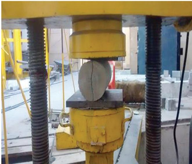
Fig. 4 Test Setup for Split Tensile test.
