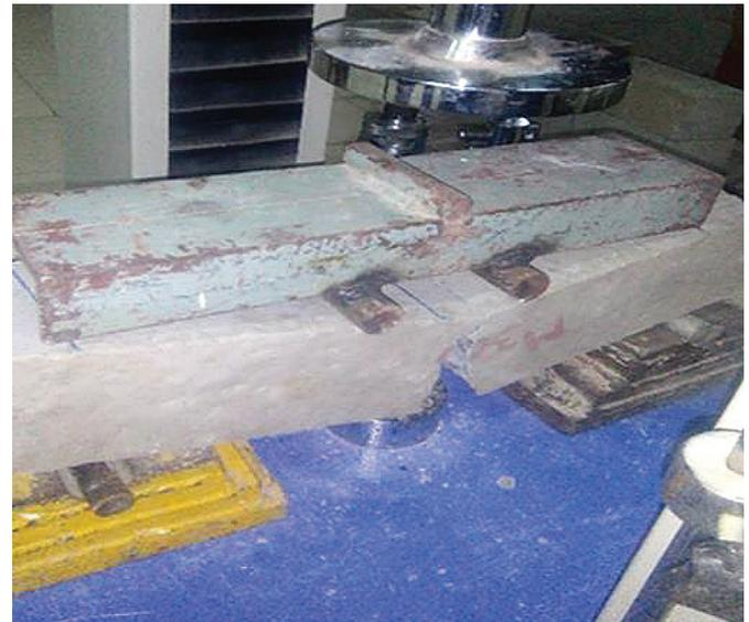
Fig. 5 Test Setup for Flexural Strength.
