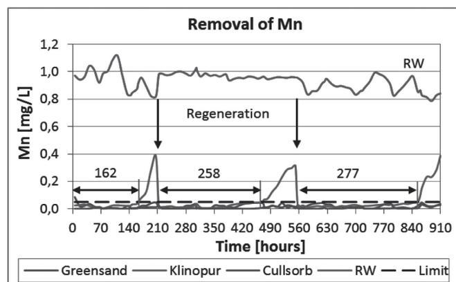
**Fig. 6** Course of removing the manganese from water.
