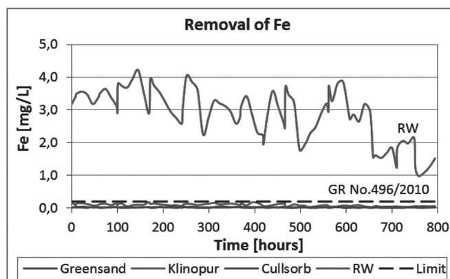
**Fig. 9** Course of removing the iron from water.
