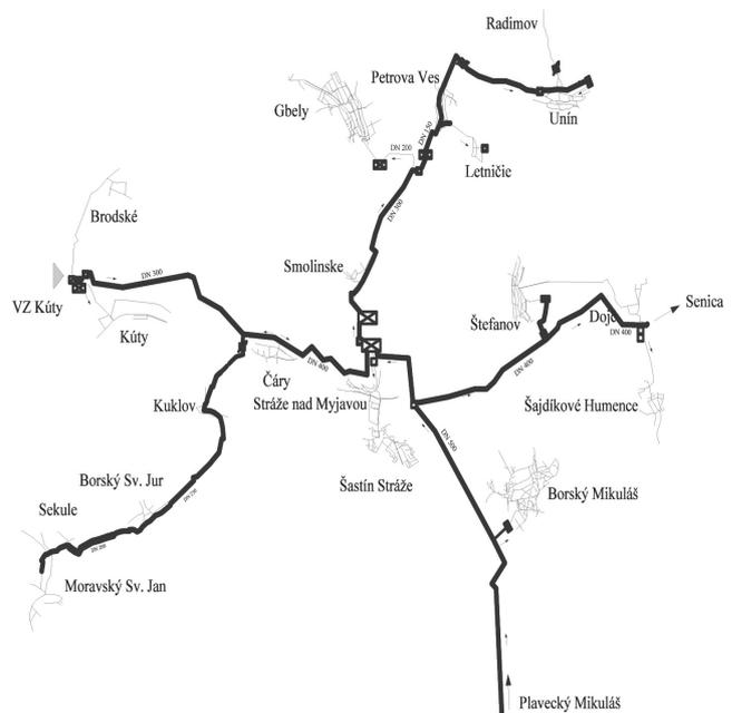
Fig. 1 Scheme of part of the Senica group water supply system.
