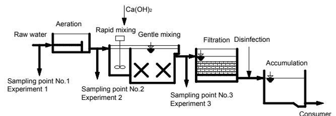
Fig. 2 Scheme of the technology of WTP Kúty and the location of the filter columns.
