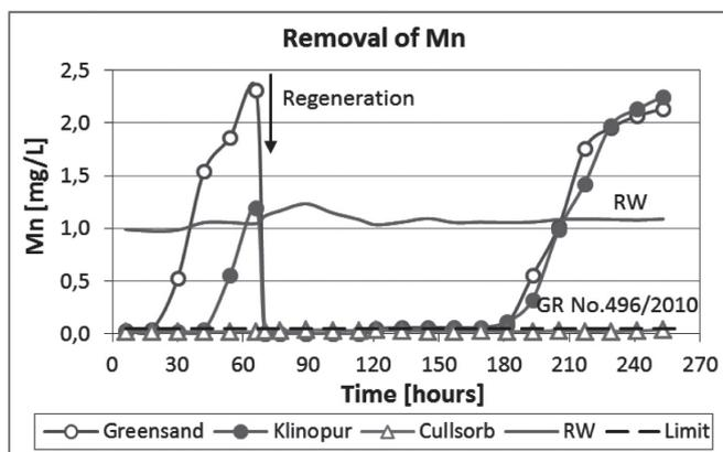
Fig. 4 Course of removing the manganese from the water.
