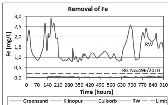
**Fig. 7** Course of removing the iron from water.
