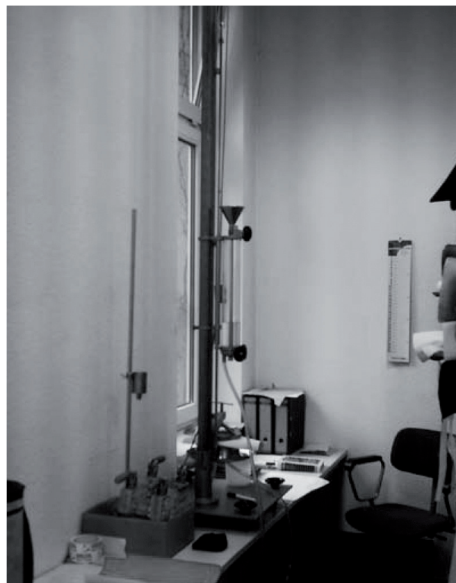
Fig. 4 View of the testing device for the measurement of watertightness by the method of a maximal water column up to 1500 mm during the test.
