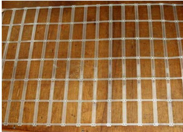
Figure 6: View of geogrid reinforcement.
