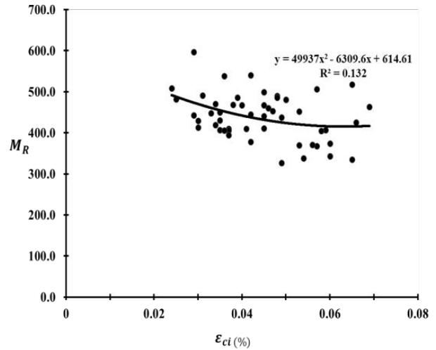
Figure 18: Relationship between  $M_R$  and crack initiation strain ( $\varepsilon_{ci}$ ).
