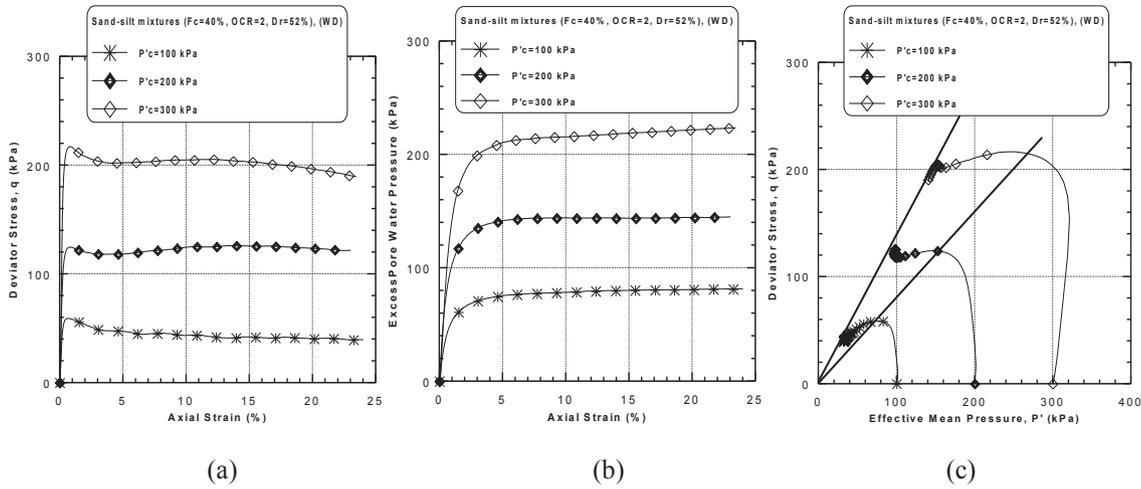
**Figure 14:** Undrained monotonic response of wet deposited sand–silt mixtures ( $F_c = 40\%$ ,  $OCR = 2$ ,  $D_i = 52\%$ ): (a) deviator stress versus axial strain, (b) excess pore water pressure versus axial strain and (c) stress path diagram.
