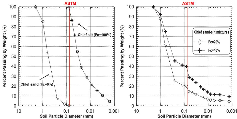
Figure 3: Grain size distribution curves of tested soils.
