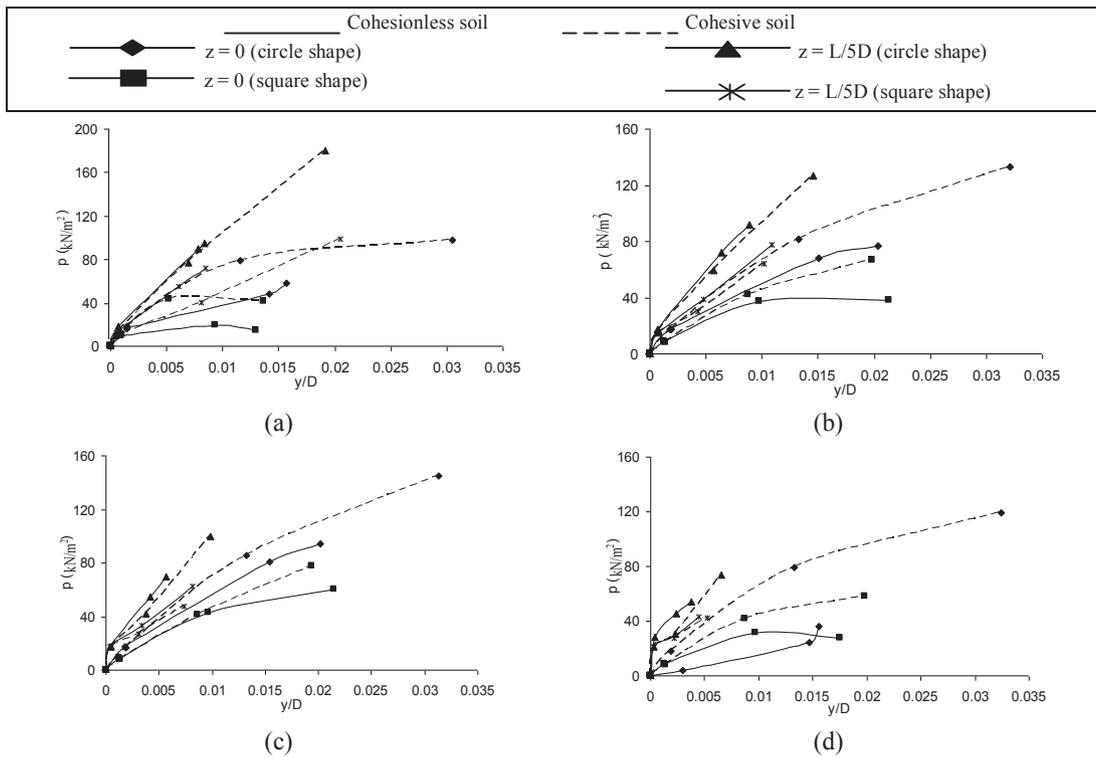
Figure 9:  $p$ - $y$  curves predicted under the effect of pile shape and pile slenderness ratio of pile embedded on both cohesionless and cohesive soils: (a)  $L/D = 10$ , (b)  $L/D = 15$ , (c)  $L/D = 20$  and (d)  $L/D = 25$ .
