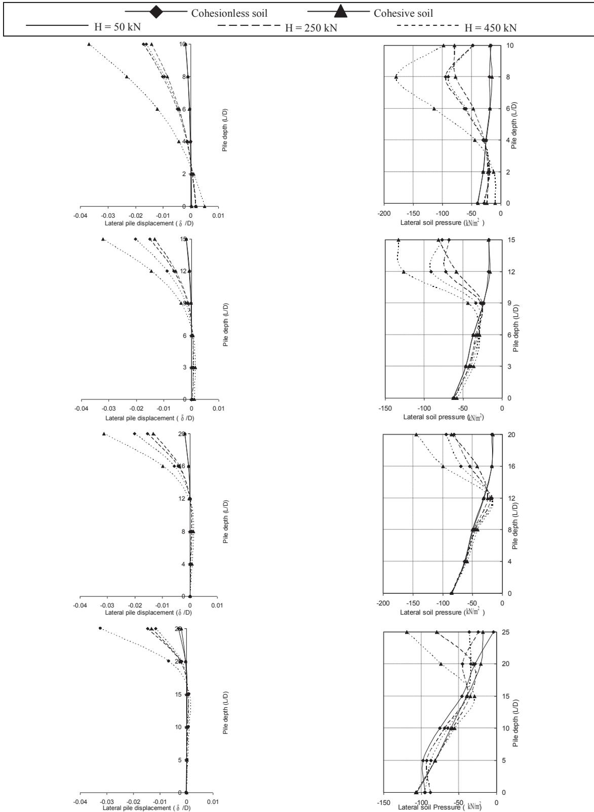
Figure 4: Influence of lateral load intensities on the lateral soil pressure distribution of pile embedded on both cohesionless and cohesive soils: (a)  $L = 10m$ , (b)  $L = 15m$ , (c)  $L = 20m$  and (d)  $L = 25m$ .
