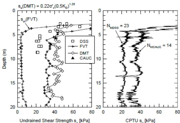
Fig. 2. Undrained shear strength data from laboratory recompression tests (DSS, CAUC) and in situ tests (FVT, DMT, CPTU) [6]
