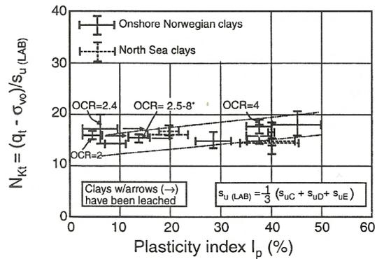
Fig. 3. A dependence between the determined  $N_{kt}$  and plasticity index [7]
