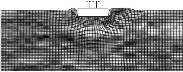
Fig. 6. A realisation of cohesion random field (lognormal)
