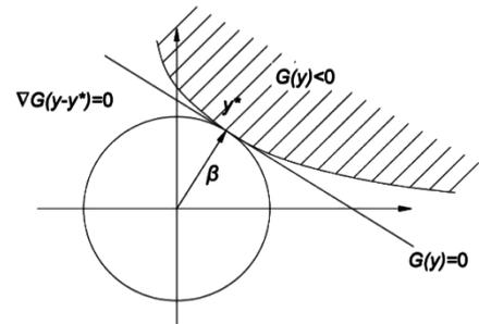
Fig. 2. Graphical presentation of limit state surface approximation according to the first-order reliability method
