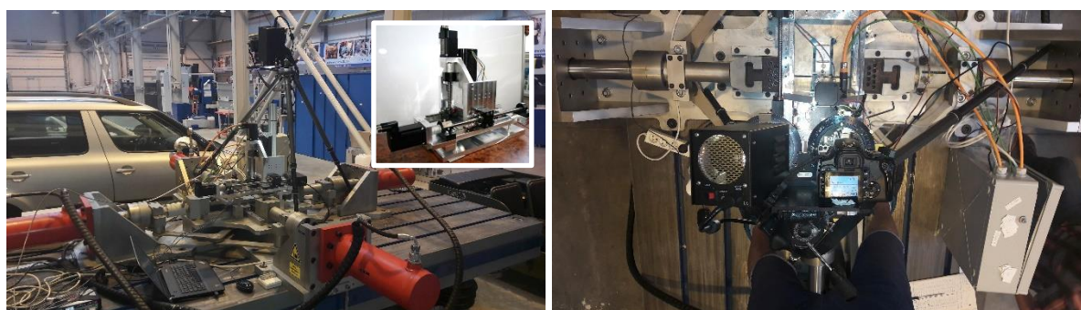
Fig. 18 Using the Photostress method for quantification of residual stress in accordance with standard ASTM E837-13a.
