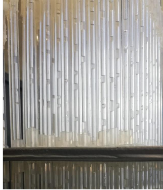
b) Detail look at the vapour bubbles and liquid plugs formed in the ML-OHPHE.
