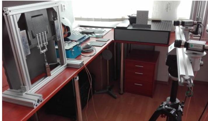
Fig. 10 Measuring string used by the measurement via DIC method.
