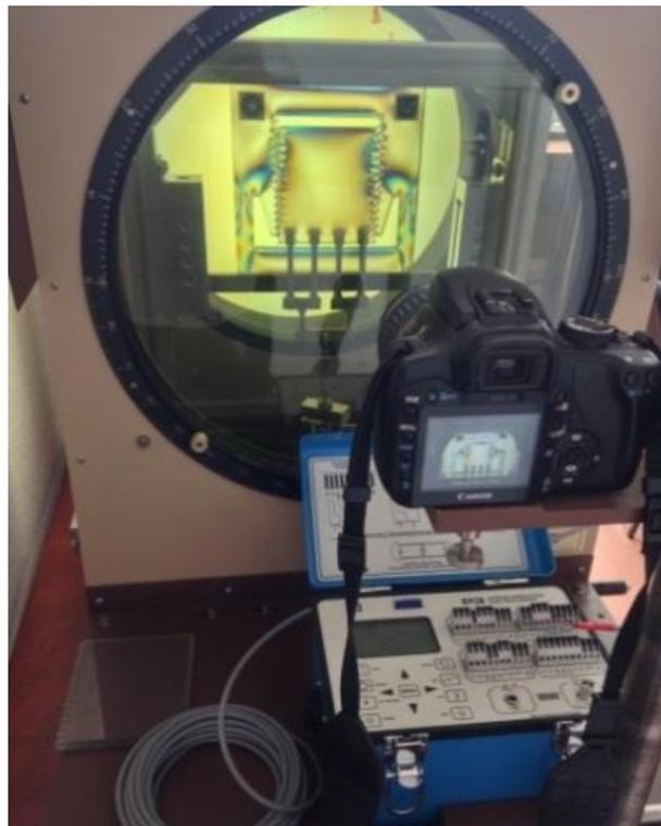
Fig. 6 Measuring string used by the measurement via transmission photoelasticity.
