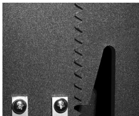
Fig. 14 Image captured by one of the cameras at a detailed analysis of the area with the notch.
