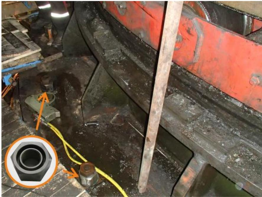
Fig. 4 Female screw M56 with a created notch used for anchoring of a casting pedestal.
