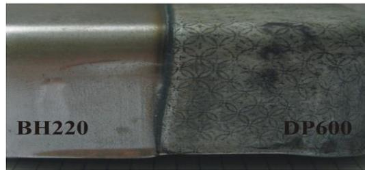
Fig. 14. Experimental weld line movement with longitudinal orientation of the weld line
