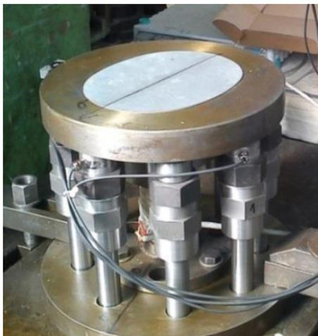
Fig. 3 Part of deep drawing tool with TWB
