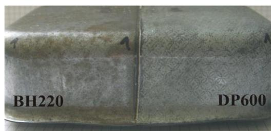
Fig. 16. Experimental weld line movement with transversal orientation of the weld line
