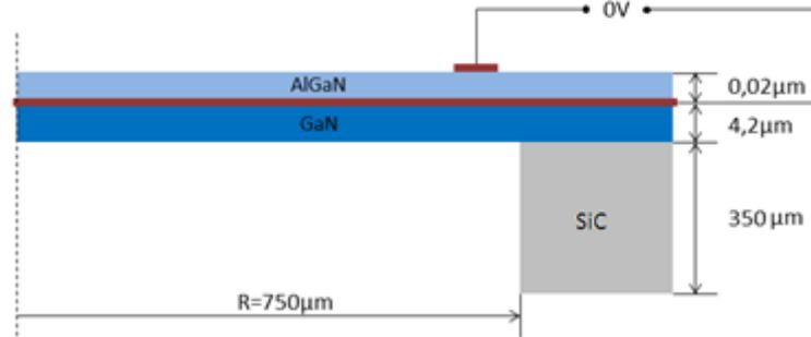
Fig. 1 Dimensions of the equivalent model of the membrane
