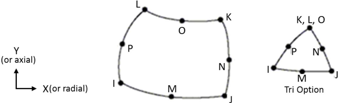
Fig. 2 Geometry of the 2-D elements PLANE183 and PLANE223 [3]
