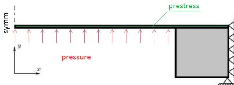
Fig. 4 Boundary and loading conditions in the model
