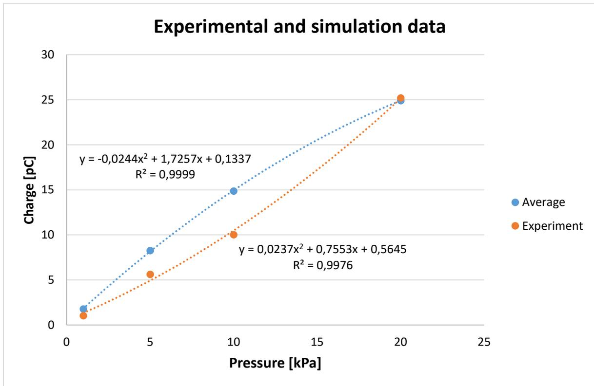
Fig. 6 Graphical representation of the average values (simulated) and experimental results
