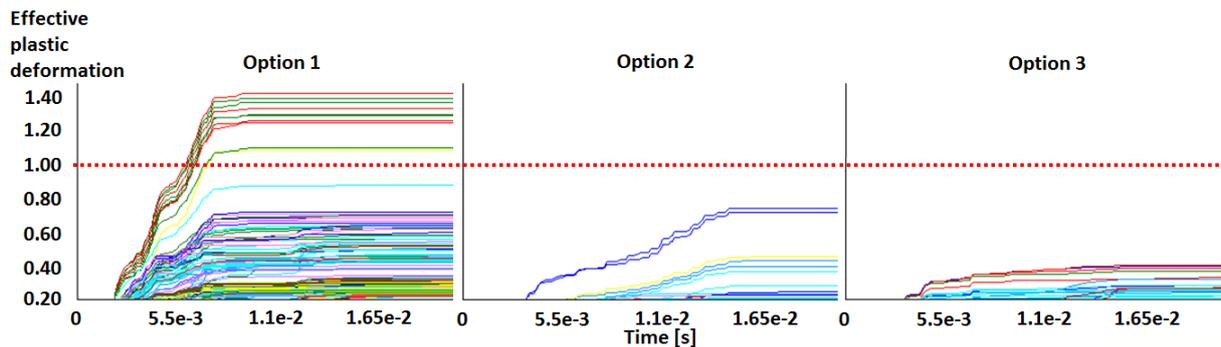
Fig. 9 Effective plastic deformation of heat affected zone over time
