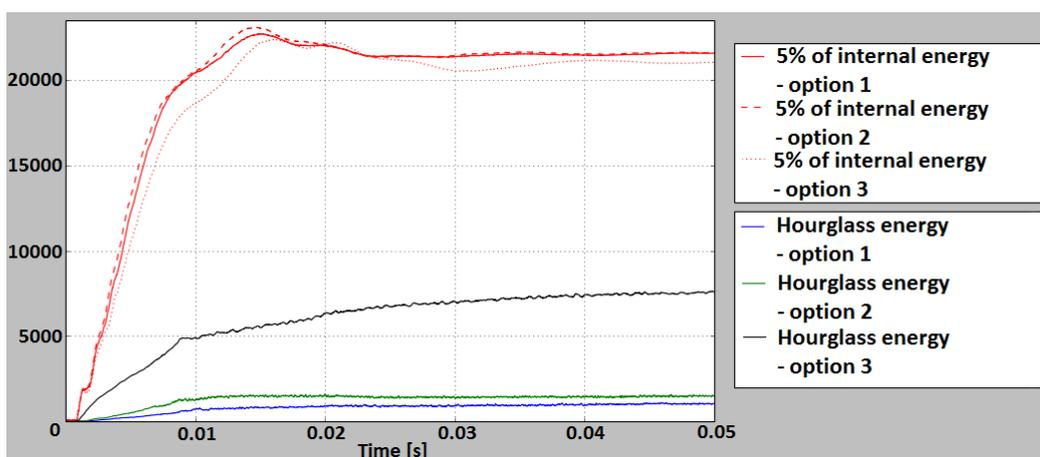
Fig. 8 Hourglass energy over time
