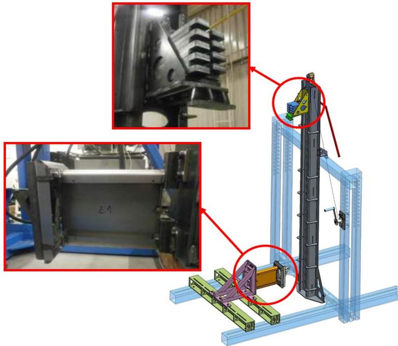
Fig. 2 Impact testing device constructed by BORCAD cz s.r.o.
