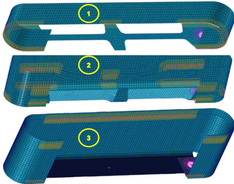
Fig. 7 Welds and heat affected zone for all three design options
