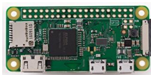
Figure 2. Raspberry Pi Zero W development board
