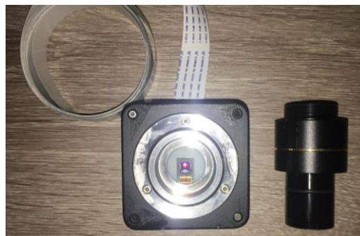
Figure 3. Optical sensor installed in the optical enclosure
