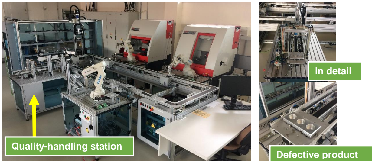
Fig. 2 Flexible Production System in process at the Research Centre with detail focused on the Quality-handling station with possibility to select defective products
