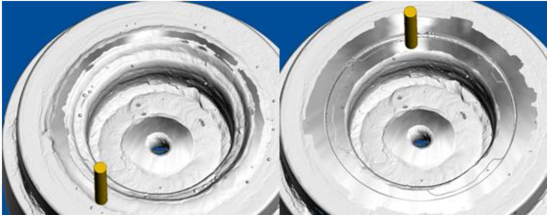
Fig. 4 Simulation of milling process according STL model
