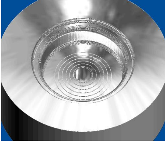
Fig. 6 Final shape after simulation of roughing with constant allowance
