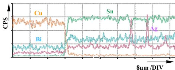
**Fig. 2** Linear EDX microanalysis of  $\text{Cu} - \text{SnAg}1.0\text{Cu}0.5\text{Bi}0.5$  solder joint interface aged at  $160\ ^\circ\text{C}$  for 24 h
