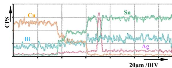
**Fig. 3** Linear EDX microanalysis of  $\text{Cu} - \text{SnAg}1.0\text{Cu}0.5\text{Bi}0.5$  solder joint interface aged at  $160\ ^\circ\text{C}$  for 360 h
