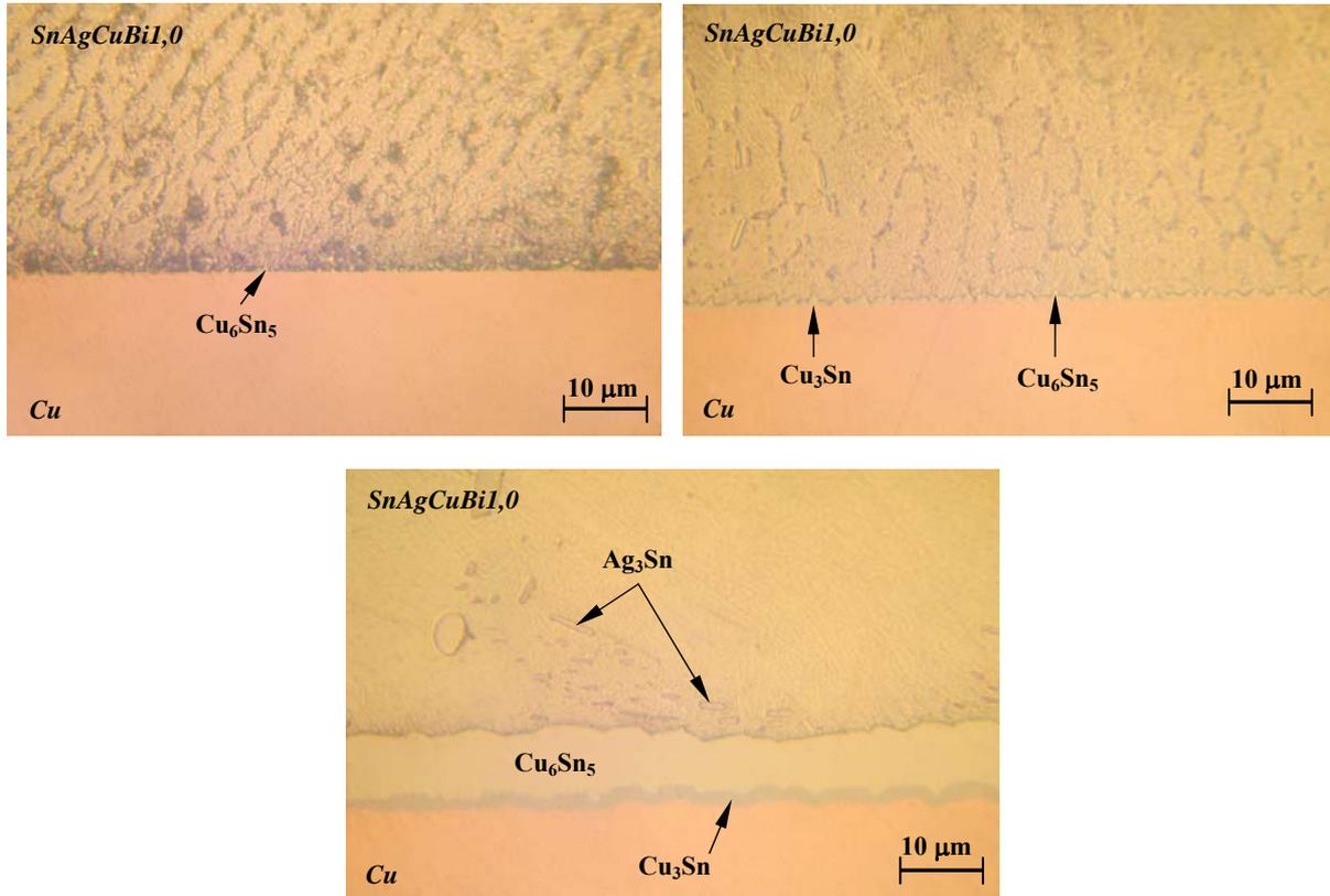
**Fig. 4** Microstructure of the interfacial area of Cu-SnAg1.0Cu0.5Bi1.0 solder joint
