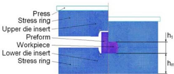
Figure 5: FE model of closed-die upsetting process.
