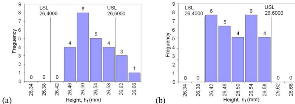
**Figure 11:** Frequency histogram of product height tolerances,  $h_1$ , for various press stiffness conditions, (a) soft press, (b) stiff press.
