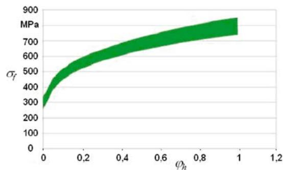
Figure 14: Scatter of flow stress for 16MnCr5 steel [8].
