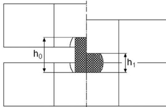
Figure 4: Closed-die upsetting process, value of relative deformation  $\epsilon_h = 0.45$ .
