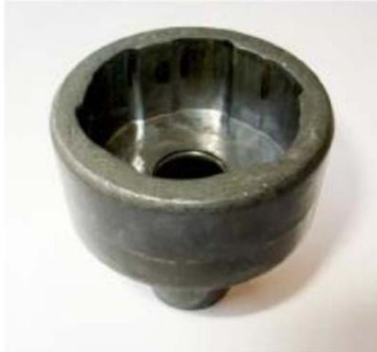
Figure 17: Clutch barrel of a starter.
