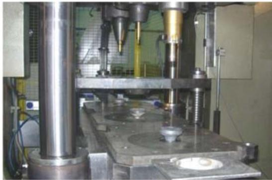
Figure 19: Three-stage tooling for barrel production.
