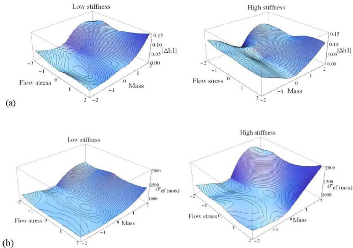
**Figure 10:** Influence of the scatter of mass and flow stress input parameters on the (a) dimensional accuracy of product,  $|\Delta h|$ , and (b) on maximal effective stress in the die,  $\sigma_{\text{eff(max)}}$  for various press stiffness conditions in the closed-die upsetting process.
