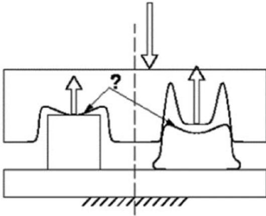
Figure 16: An example of a two-stage forming process.
