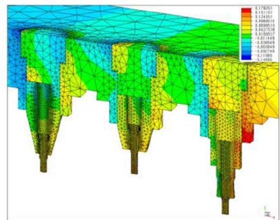
Figure 23: A relative displacement between the upper tool and press bolster.
