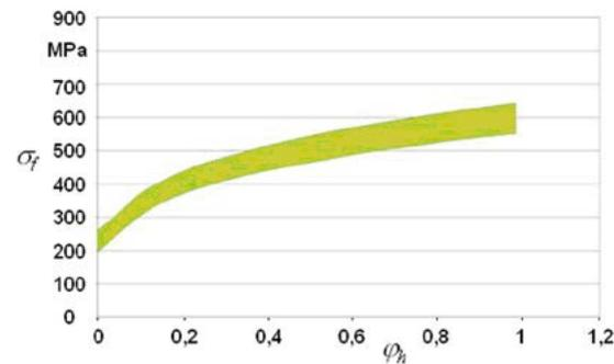
Figure 6: Scatter of flow stress QSt 32-3 steel [8].
