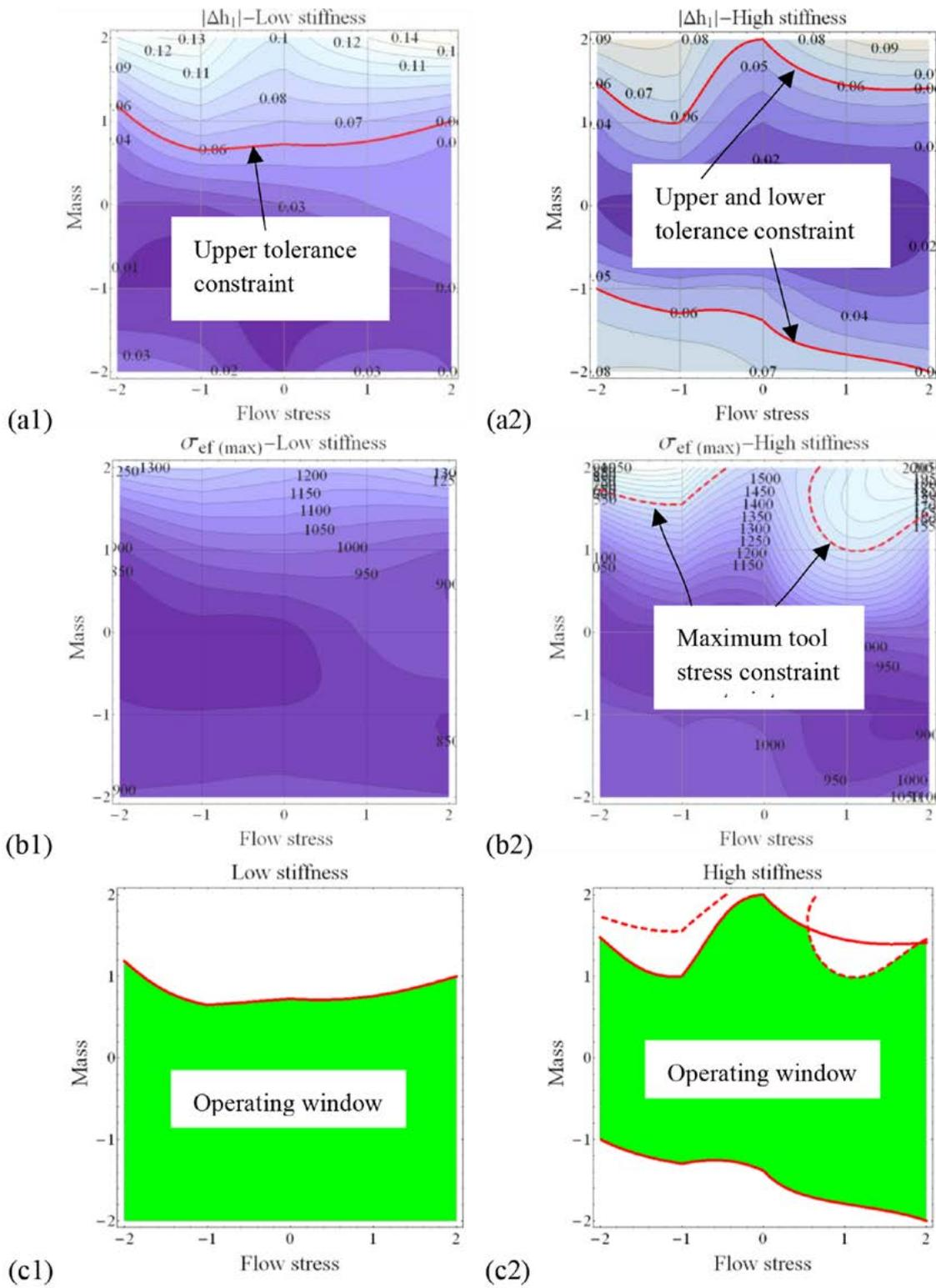
**Figure 12:** (a1 and a2) feasible region for the product height ( $h_1$ ) accuracy, (b1 and b2) feasible region for maximum effective stress in the die, ( $\sigma_{ef(max)}$ ), and (c1 and c2) operating window for the closed-die upsetting process for low and high press stiffness.
